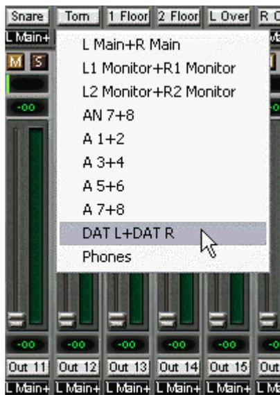
The hardware outputs (third row) can be edited in the same way. In this case, the names in the routing drop down menus will change automatically. Additionally the names in the drop down menus of the Monitor section will change as well.
