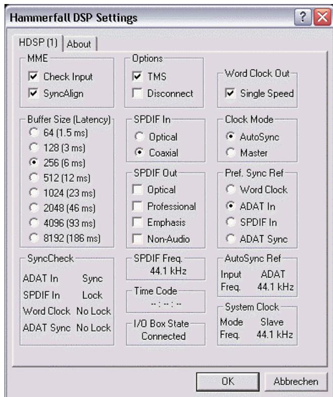
Thanks to its AutoSync technique and lightning fast PLLs, the HDSP is not only capable of handling standard frequencies, but also any sample rate between 28 and 103 kHz. Even the word clock input, which most users will use in varispeed operation, allows any frequency between 28 kHz and 105 kHz.
