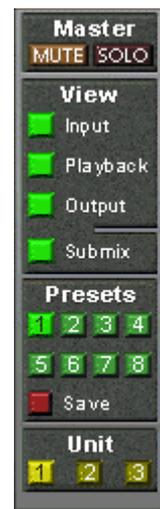
Instead of single presets a complete bank of (8) presets can be loaded at once. Advantage: The names defined for the preset buttons will be stored and loaded automatically.
