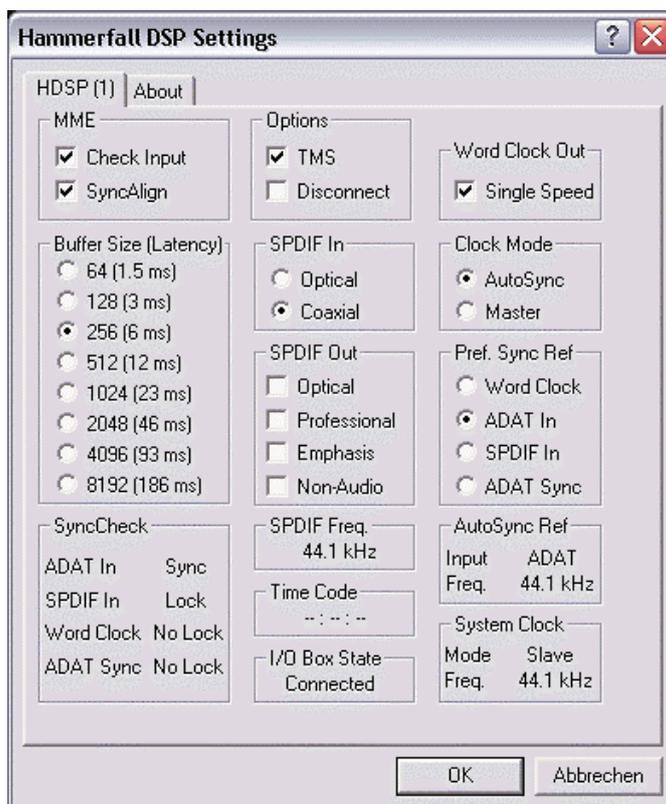
*SyncCheck* indicates whether there is a valid signal (Lock, No Lock) for each input (Word Clock, ADAT, SPDIF), or if there is a valid *and* synchronous signal (Sync). The *AutoSync Reference* display shows the input and frequency of the current sync source.
