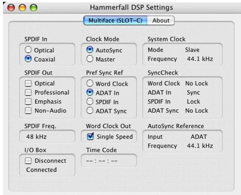
In practice, SyncCheck provides the user with an easy way of checking whether all digital devices connected to the system are properly configured. With SyncCheck, finally anyone can master this common source of error, previously one of the most complex issues in the digital studio world.
