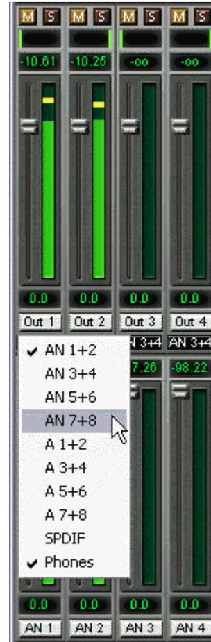
Often signals are stereo, i. e. a pair of two channels. It is therefore helpful to be able to make the routing settings for two channels at once. Hold down the Ctrl-key and click into the routing field of Out 3. The routing list pops up with a checkmark at 'AN 3+4'. Select 'AN 7+8'. Now, Out 4 has already been set to 'AN 7+8' as well.
