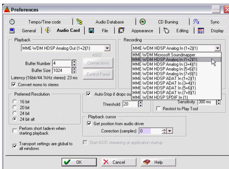
The HDSP system's ADAT optical interface allows sample rates of up to 96 kHz using a standard ADAT recorder. Single-channel data at this frequency requires two ADAT channels, achieved using the *Sample Multiplexing* technique. This reduces the number of available ADAT channels from 8 to 4. Under Windows MME, channels are routed to ADAT devices in double-speed mode as follows:
