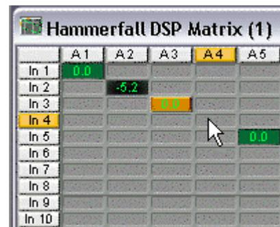
To maintain overview when the window size has been reduced, the left and upper labels are floating. They won't leave the visible area when scrolling.
