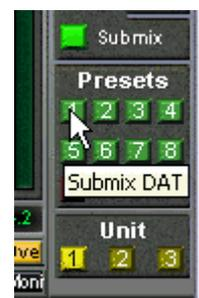
The preset button names are not stored in the preset files, but globally in the registry, so won't change when loading any file or saving any state as preset. But loading a preset bank (see chapter 28.8) the names will be updated.
