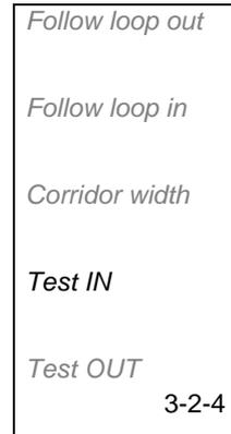
When the function is selected the mower will immediately follow the boundary wire, guide 1 or guide 2, depending on which one it finds first, in to the charging station. If there is a passage and the mower can not run through it, the *Corridor width* value is set too high. When *Test IN* is activated, the mower runs at the greatest distance from the wire that the selected corridor width permits.
