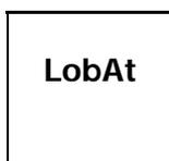
It means that the battery is low voltage. Under such condition, the Datalogger function is disable.
