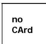
It means that the SD card is not plugged into the meter.
